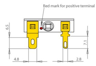
Thickness, both terminals: 0.5mm Terminal plating: Gold
