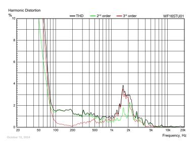
Measuring conditions, distortion Driver mounting: 16 lit. sealed cabinet Input voltage: 5.3 VRMS Smoothing: 1/12 oct.
