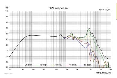
$\underline{\textbf{Important!}}$  Please observe that graphs on the left side of this page and the below text files for download are actual measurements of the drivers measured in infinite baffle and without any enclosure. Measuring the drivers in a finite baffle (like the baffle of most speaker cabinets) and in any size of enclosure will lead to different response curves.
