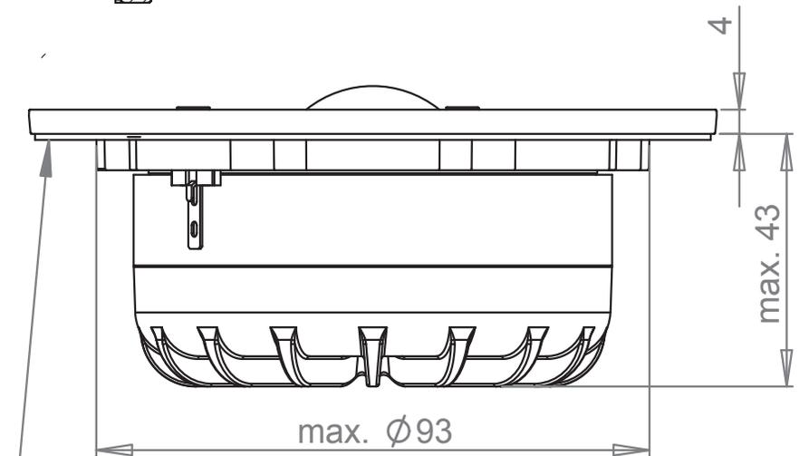
EVA gasket attached on the rear side of face plate
