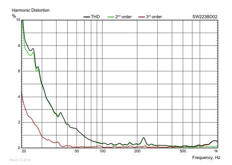
Measuring conditions, Harmonic Distortion Driver mounting: In sealed, heavily stuffed enclosure, internal volume 28 lit. Microphone distance: 0.5 m Input signal: Stepped sine wave, 8.95 VRMS (SW223BD02) / 12.65 VRMS (SW223BD03) Smoothing: 1/12 oct.
