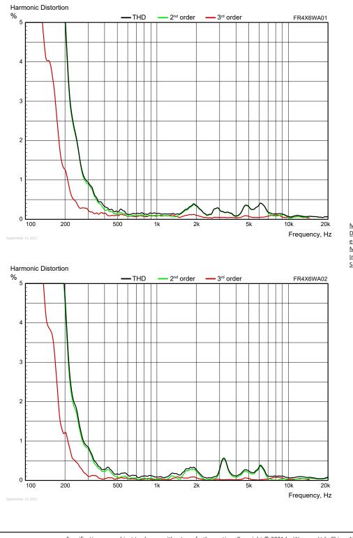
Measuring conditions, harmonic distortion Driver mounting: In sealed, heavily stuffed enclosure, internal volume 1 lit. Microphone distance: 0.5 m Input signal: Stepped sine wave, 2.45 VRMS Smoothing: 1/6 oct.
