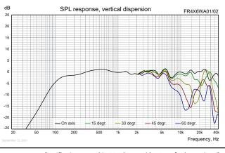
Download FR4X6WA01 on-axis SPL response as .txt file Download FR4X6WA02 on-axis SPL response as .txt file <u>Measuring conditions, SPL</u> Driver mounting: Flush in infinite baffle, back side open (no cabinet) Microphone distance: 1.0 m
